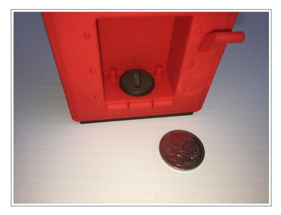
Then use a coin in the pin slot and turn the pin 90 degrees which will then lock the containment unit to the base.
