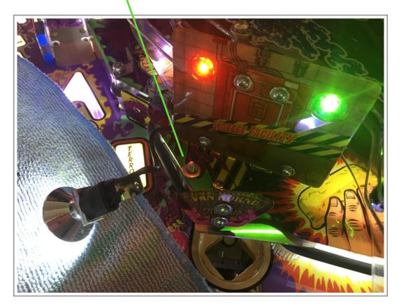
Now remove the Storage Facility Plastic from 2 small 90 degree metal brackets.
