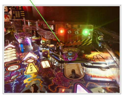
Remove the spotlight from it's post as this gives you better access to the screw for the plastic removal and new mod installation.
