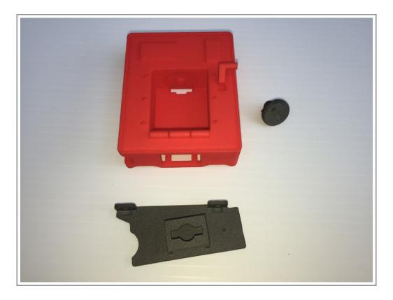
Slide the top over the base and then drop the pin into the hole.
