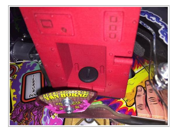
Then use a wide thick blade screw driver to turn 90 degrees which then locks the cabinet to the base.
