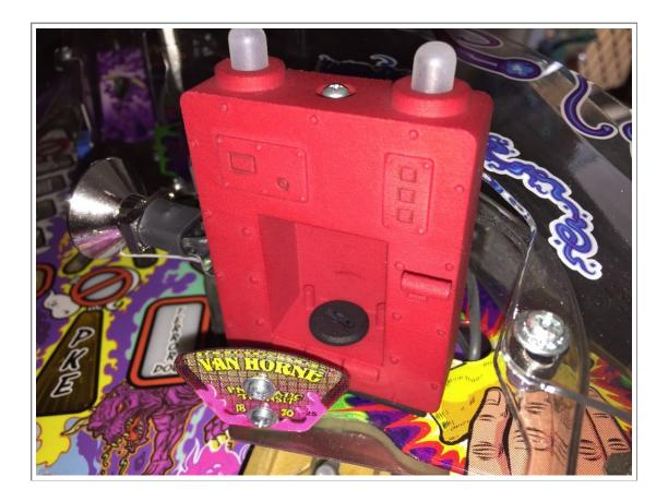
Also not in the above photo 2 pins behind the locking pin - the cabinet door has 2 x arms coming off with 2 holes in them. The cabinet door simply slides over these pins until the bottom of the door is very close to the cabinet hinge.
