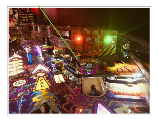
Remove the spotlight from it's post as this gives you better access to the screw for the plastic removal and new mod installation.
