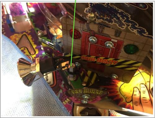
Remove the spotlight post from the top of the plastic - ensure not to loose any of the washers.
