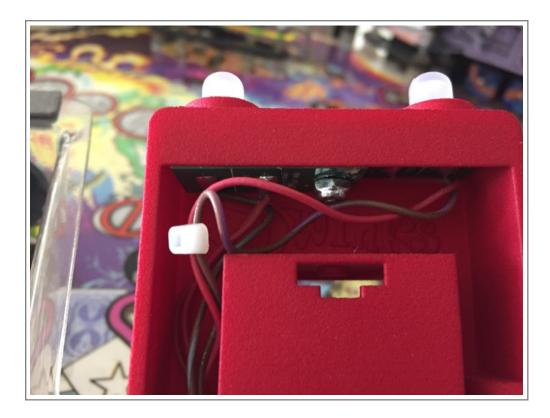
You will notice a recess inside the cabinet this is for an extra Comet Star Post LED board to add extra lighting if desired and connect to a feature globe for extra effect - Note provided with the mod. Use a dab of hot glue to hold the board in place.
