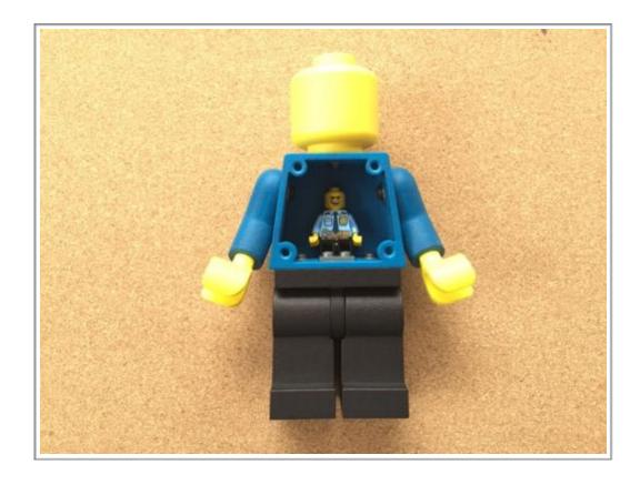
Lastly you can install the chest plate with the pins to the matching aligned holes in the chest. This component is not perfect and a tad loose. We plan to design a flip down chest plate on the version 2. And unfortunately you do see the pin marks on this part.
