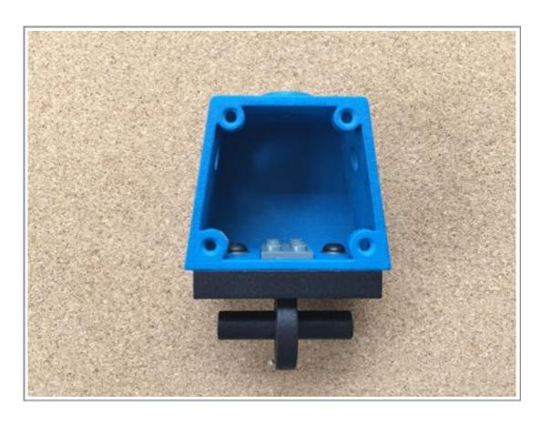
Next is fitting the head which also a little tricky as bolted from within the body up into the neck of the head.
