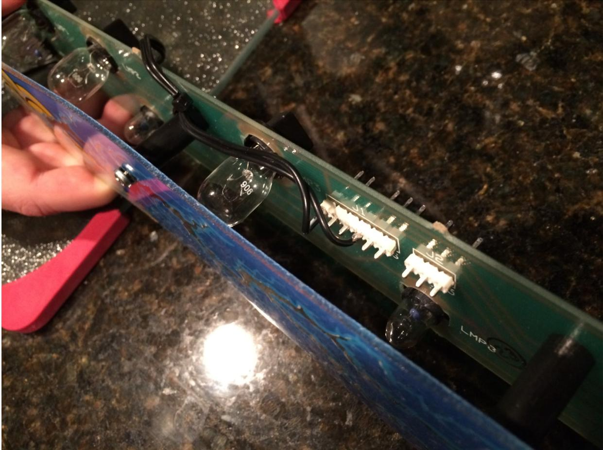
I soldered a connector wire to the back of the 6 pin header, used a zip strap to connect the wire to a post as stress relief, and then ran the wire down to input 2 on the PIG 2.
