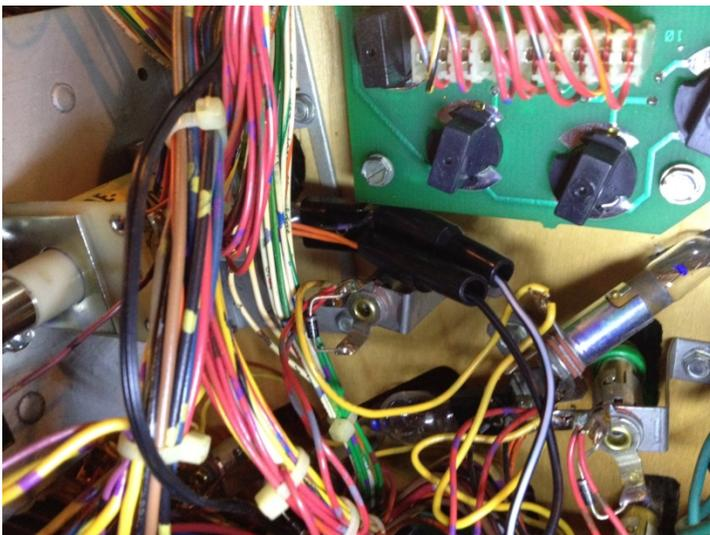
Last, using alligator clips, I connected the "drop target flasher" to Input 3 on the PIG 2.
