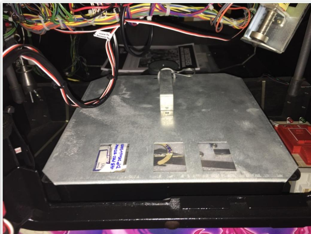
Now take the modded Coin Door Plate with the Coin Box Mount fitted and slot into the very LHS slot and push it back and it will just rest there has it has a 2.5 degree lean back designed into the bracket and you are good to start enjoying your mod. You can always add a blob of hot glue or a piece of tape to stop the bracket from sliding forward.
