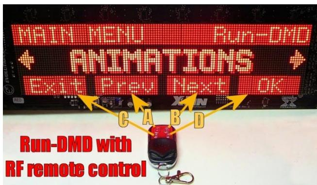
Run-DMD will remember where you exited the menu system and re-enter at the same main menu level to make repeated tests of the effects of a setting easier.
