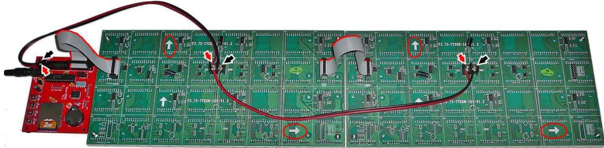
1. Install the included CR2032 battery in the holder on the Run-DMD. (During startup the Run-DMD will indicate if this battery needs replacing. The first power up after installing/replacing the battery Run-DMD will still indicate "Replace battery" to alert you that the clock settings have been lost and needs to be adjusted.)
