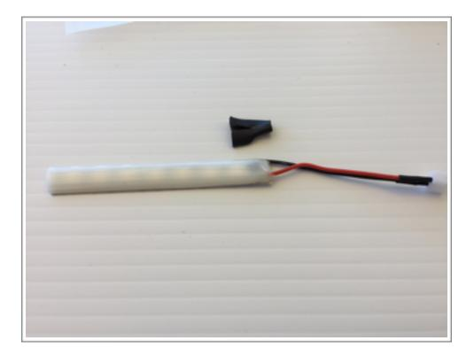
**Step 4** - Insert the now 7SMD into the back of the housing with the wiring coming out of either the <u>S</u> or the <u>r</u> end. The choice of end is yours but will be determined when and where you choose to install the mod and hiding the wiring. (sorry for the photo shape change).
