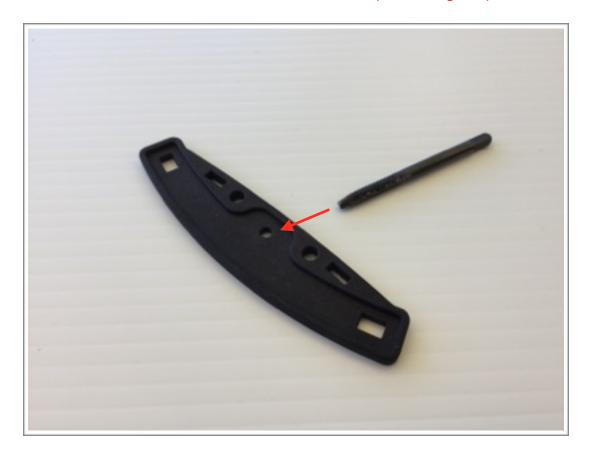
**Step 4** - Time to insert the resin insert into the sign housing in which there are 2 approaches and each one has their pros and cons.
