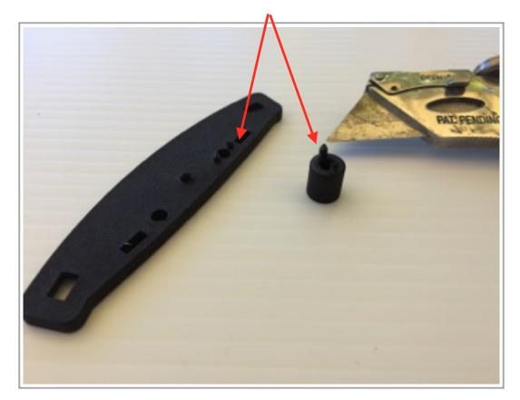
**Step 3** - Tap the centre hole of the housing as this is used to hold down the housing top. *You could drill out and fit a nut on the underside to avoid purchasing a tap.*
