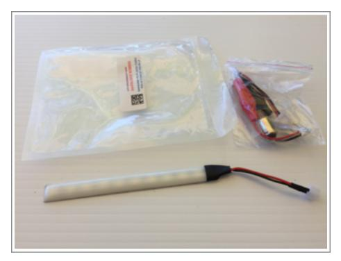
**Step 2** - The strip needs to be trimmed down to 7 SMD's to fit into the Housing and while the clear strips would be easier to perform the trim, the frosted strip gives you a better look once installed. Comet Pinball supply the below image and while is is very handy it does have a slight mistake. At the end of the strip the SMD and Resistor are flipped around which can through you off as you will notice 2 black dots close together. Remove up to here:
