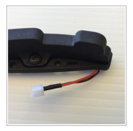
**Step 3** - Install the extension lead to the sign and also the matrix bulb and it is ready to test and then install into your game.
