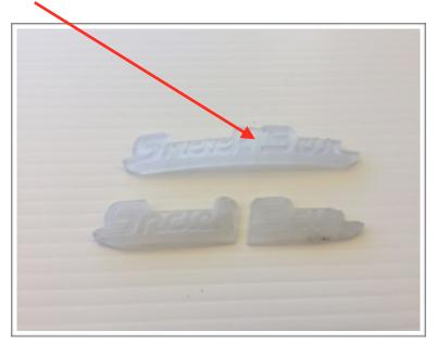
ii - slide the <u>Snack</u> part in and using a knife press from the back until the letters of the resin insert are flush with the housing front face.
