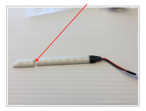
**Step 3** - Remove the heat shrink so the remaining 7 LEDs strip can fit into the housing behind the resin insert.
