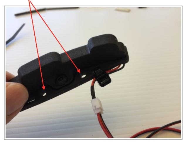
Pass a bolt / screw down through one of these and use the detached post or another pinball post to anchor the mod to the game. There are also 2 slots in the back for cable fastening to neaten it up.
