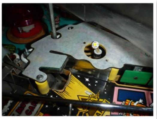
TIP: since the Snackbar mod is significantly taller than the original playfield plastic, I suggest purchasing an LED bulb with a flexible extension (as shown in the image) to that you can direct the light into the new dome.
