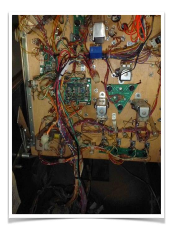
• Using a couple of zip-ties, fasten the blue inverter box to the existing harness that runs below the snack bar scoop (as shown in the photo).
