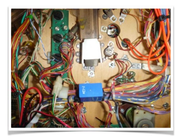
• Due to the inverter design since batch 2 (roughly production mod No: 25 and onwards) I now double cable tied the wires exiting the inverter to the inverter - leave these in place when installing to avoid wires pulling out of the inverter.
