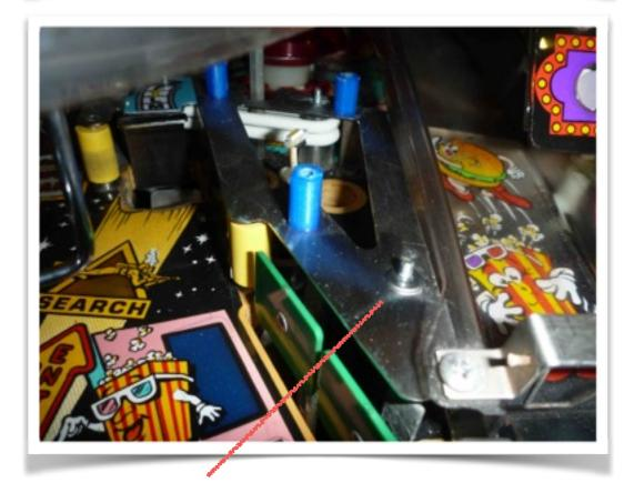
**NOTE**: Using one of the included washers, place it on the post near the two right-side stand up shown with the red line targets before securing the SS plate. The reason is if you don't the nut will not bind well to the flat. You want to make sure that the SS plate is secured well to the post before proceeding.
