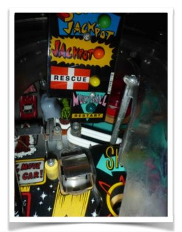
Remove the 2 5/16" nuts and the phillips screw securing the original Snackbar plastic in place. My apologies this photo has a brand new uncovered plastic to show what is original and installed.
