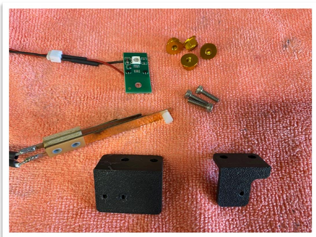
Then you will need a length of 2 core wire / cable for the switch. You will need a 900mm / 36 inch cable and bear back both ends and treat with solder and then solder one end to your purchased leaf switch.
