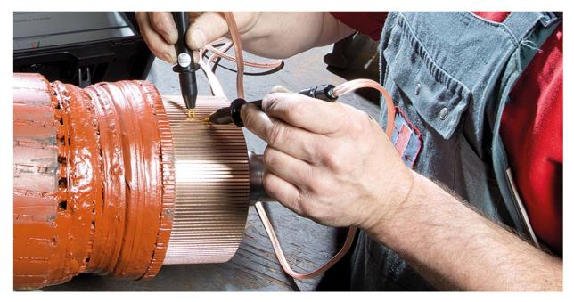
• Resistance test, moving from bar to bar with 4-wire test probes.
