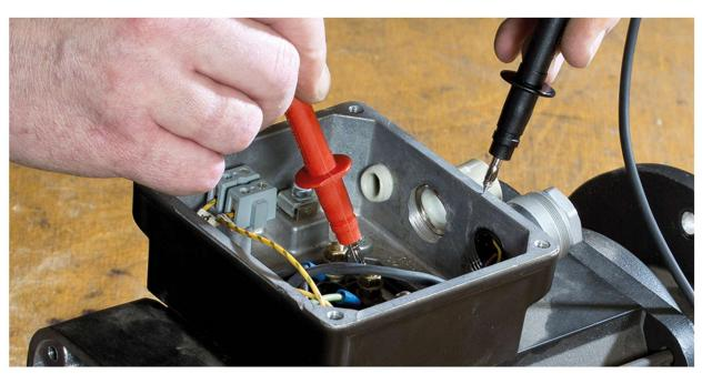
• Testing with test probes to find faults to frame and phase-to-phase faults.
