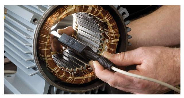
$\bullet \ \ \text{Turn-to-turn fault detection of a stator with a test probe, moved from slot to slot through the entire stator.}$
