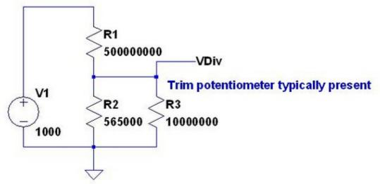
The reason that a special high voltage resistor is required is manifold. Reasons include voltage rating, wattage and other reasons. High voltage resistors may be physically very long. Length helps to minimize the effects of surface leakage currents, or provide a less severe voltage gradient across the element. Also, they may comply with design criteria called voltage
