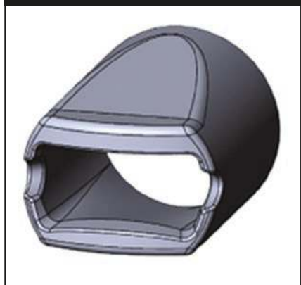
Figure 3: the Monster Nozzle has a larger inlet and no turning vanes
