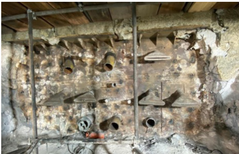
A fan jet nozzle with a focus blast capable of moving clinker further away helps maintain better control of snowmen.
