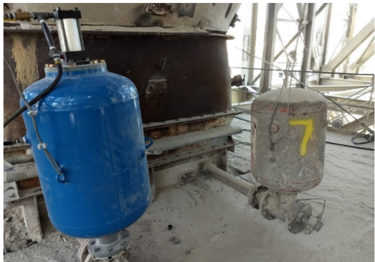
Figure 4. Bigger can be better. The air stored in an air tank is cleaning energy.
