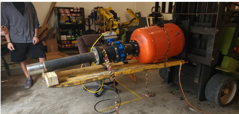
Figure 8. Dracyon's Protector Valve (butterfly valve) can be used to combat the problem of false air.
