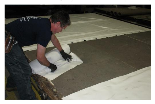
4. Using a hot-air gun, weld the last piece of membrane to itself to help the roll stay together.
