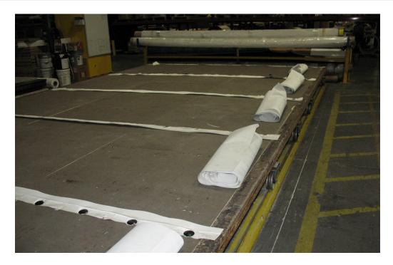
5. All membrane must be neatly stacked inside a box and secured to a pallet for shipping.
