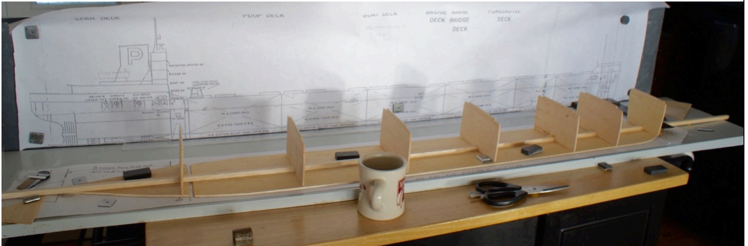
The laying of the keel...and lots of planning...the order of build is critical to having a successful end product and quality model.
