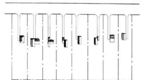
Multiple driveways impact road function.
