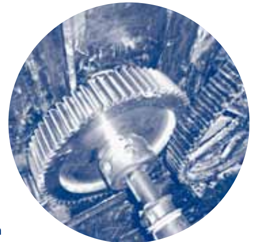
New gearing on the Lime Transfer Elevator, which is part of the corrosion control process
