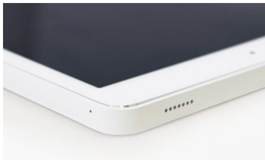
opening for the microphone and speakers
