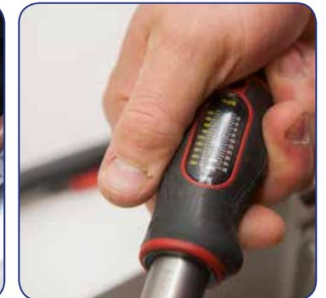
Terminals can then be clamped using a torque driver to the appropriate torque setting. If connecting pre-lugged cable the same principal applies.
