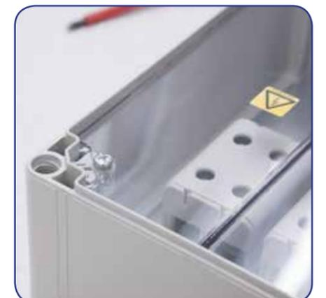
Internal shrouds are to be refitted. These are secured in place with captive fastening to prevent loss on-site. The shroud provides a segregation between terminals within the box.
