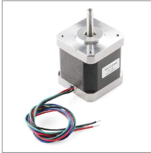
FIGURE 6. Sparkfun Electronics 400 steps/rev 68 oz-in stepper motor, the selected stepper motor to control linear translator motion.
