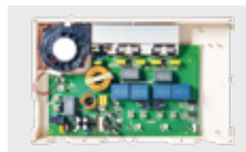
HALF BRIDGE TWO BURNER MAIN BOARD
