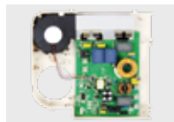
HALF BRIDGE ONE BURNER MAIN BOARD
