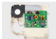
BASIC ONE BURNER MAIN BOARD
