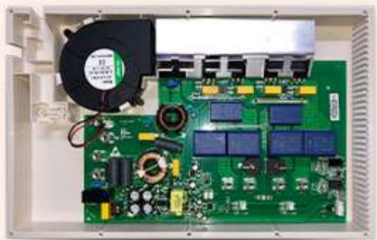
HALF BRIDGE TWO BURNER MAIN BOARD
