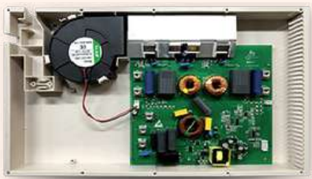
BASIC TWO BURNER MAIN BOARD
