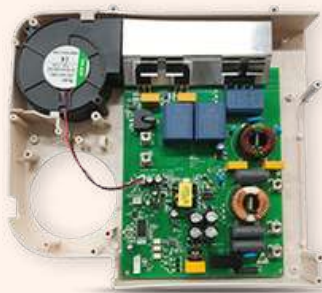
HALF BRIDGE ONE BURNER MAIN BOARD
