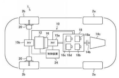
A recent patent for a "vehicle drive system" shows a mild hybrid installation with the rotary engine mounted behind the front axle, connected to a 33-hp electric motor which then sends power via a propshaft to a rear transaxle transmission. This arrangement means that the e-motor could provide useful torque-fill for the rotary at lower engine speeds. Two further electric motors of 23-hp apiece drive the front wheels and
