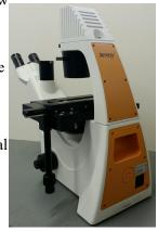
Standard with 10X eye pieces, Φ 22mm. inclined 45°; phase telescoping eyepiece, Infinity Plan objectives below, dust cover, spare fuse, power cord and anti-microbial treatment on frame, head.
