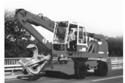
First hydraulic cab elevation
