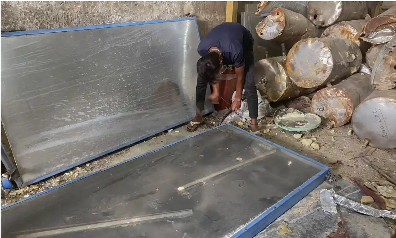
Tayyab dismantles a roof-top solar panel for heating water at his workshop in Bengaluru. The recycling is largely done by hand or with crude tools. Photograph: Flavia Lopes
