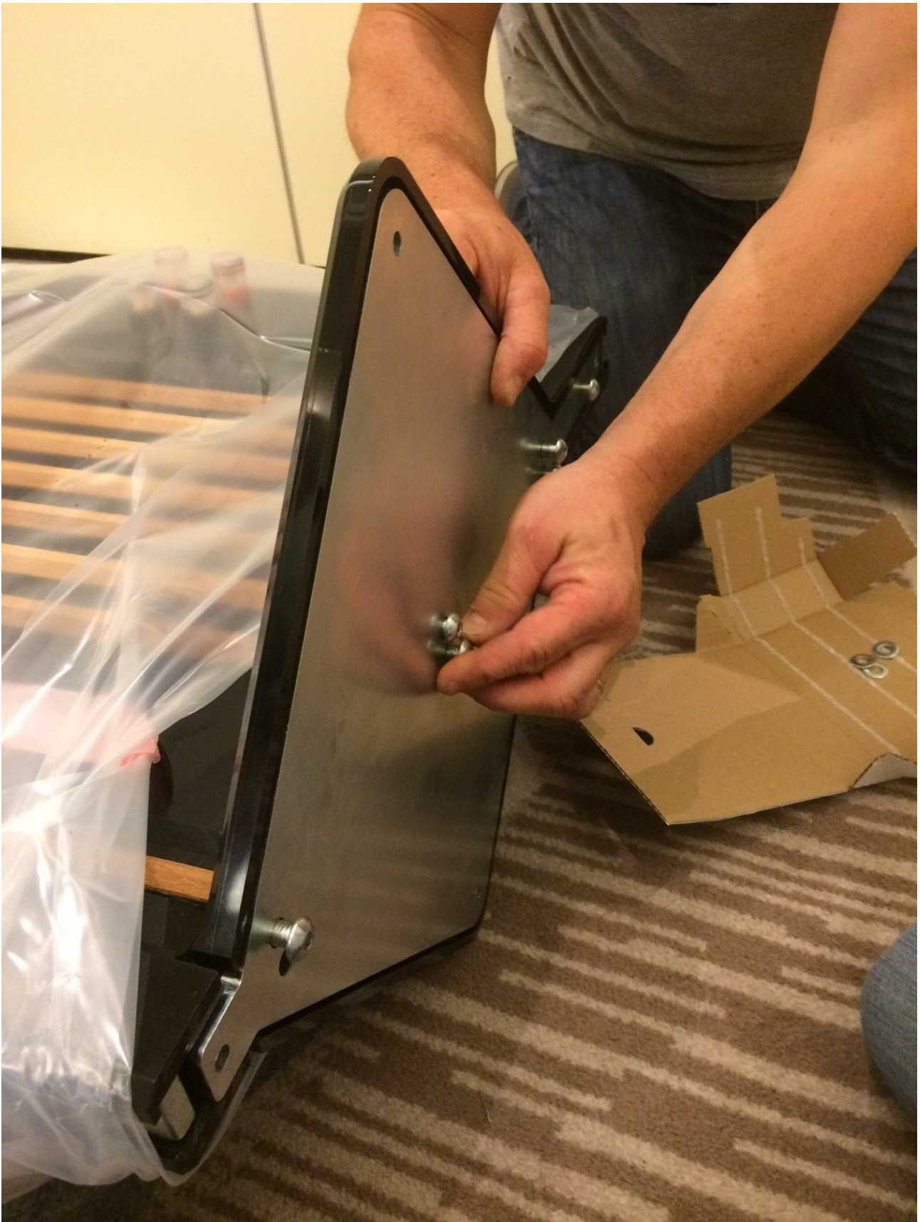
Photo 6 – Add the other screws making sure they find the hole in the washer at the inside (outside washers missing here but recommended)
