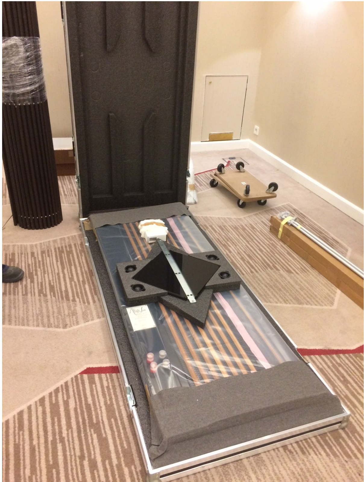
Photo 2 - Open the top of the flight case, please notice the protective grey lip that prevents touching the aluminum profile when pushing the speaker out of the edge
