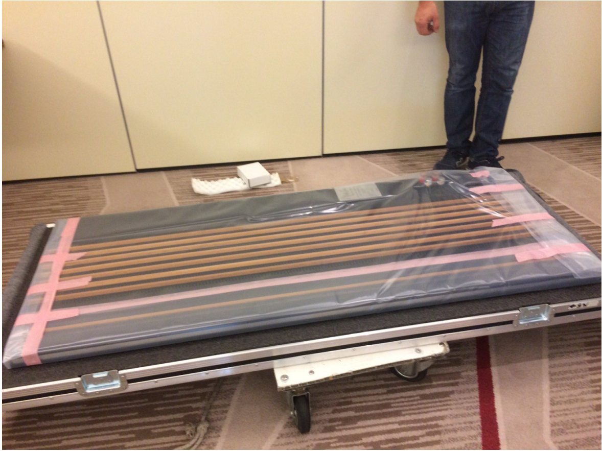
Photo 1 - Always keep the other flight case under the one you are opening to reach the right height (or leave something strong under it with about 20cm height)
