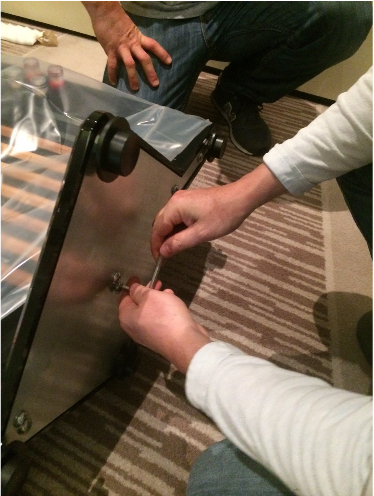
Photo 7 - Tighten the screws applying a high torque (recommend 40-50Nm if you have a torque limiter) and screw in the levelers (without cup and ball)
