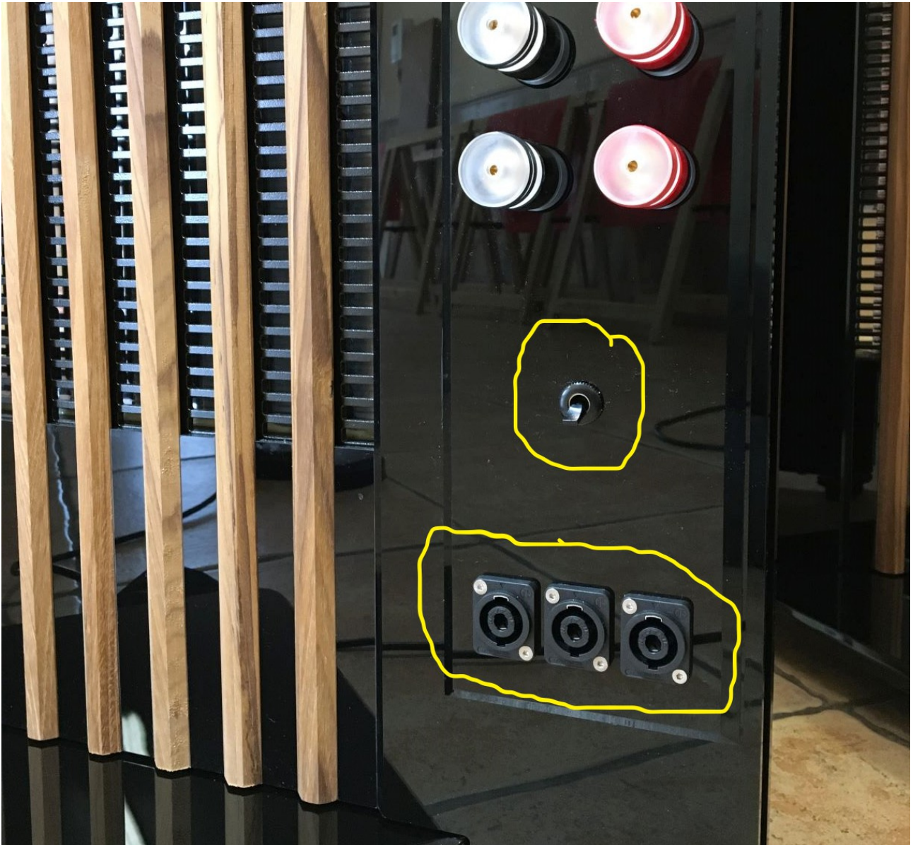
Photo 10 – Switch in the bypass position (Botticelli X) and 3 Neutrik® SpeakOn® connectors
