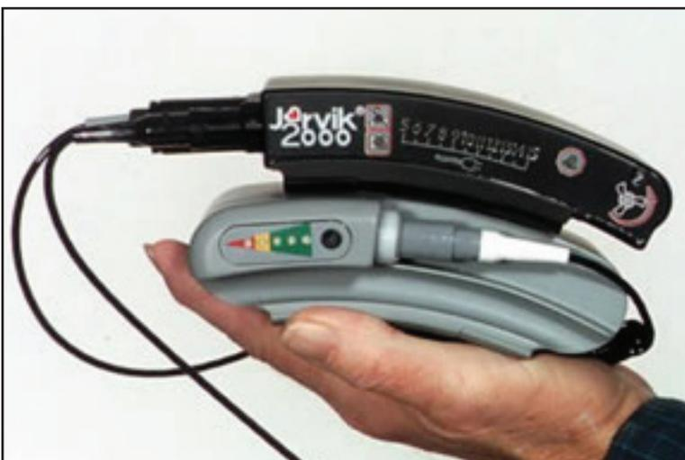
**Controller attached to the portable Li-ion battery.**
