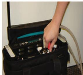
**Step 2:** Depress metal clip(s) to disconnect the pneumatic lead(s) from the TLC II Driver.
