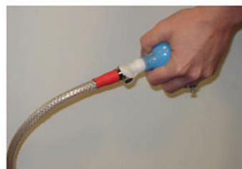
**Step 4:** Squeeze hand pump(s) once per second. Use your foot if necessary.
