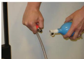
**Step 3:** Connect the hand pump(s) to the pneumatic lead(s).
