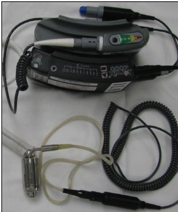
Cables are uniquely color-coded and keyed so that they cannot be mis-connected. Abdominal cable (driveline) connectors are black; power connections are gray or white.
