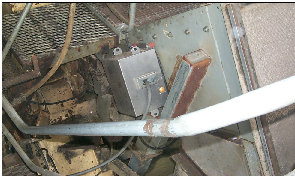
Fig. 1—System scan head mounting on the final mill exit chute.
