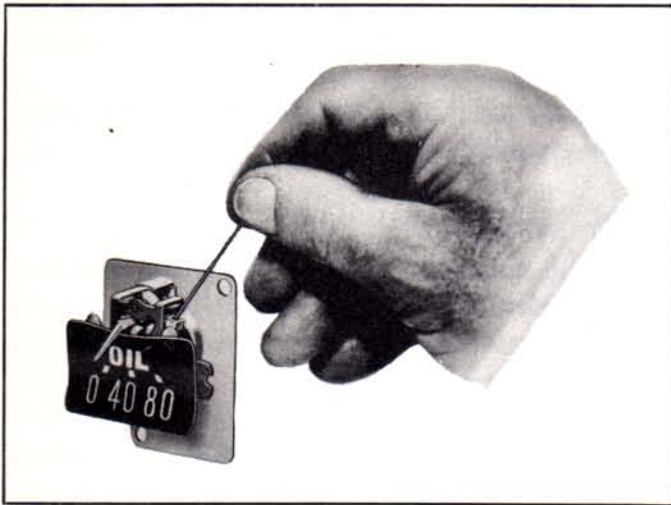
FIGURE 205—ADJUSTING THE ELECTRIC OIL GAUGE. A stiff wire placed in the "U" shaped bracket at the top of the pole shoes can be used to move the poles toward or away from the armature and increase or decrease the effect of the winding on the armature.
