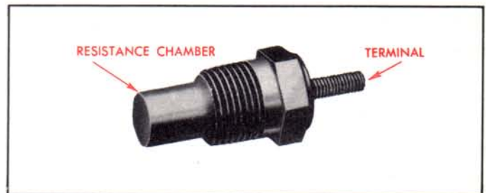
FIGURE 207—ELECTRIC TEMPERATURE GAUGE (ENGINE UNIT). A thermistor is used in this unit which decreases in resistance as its temperature rises. It is connected from the terminal to ground and controls the current flowing in the variable field circuit.
