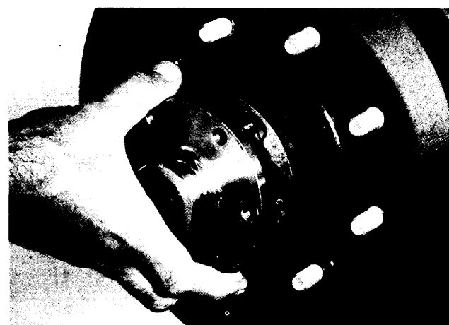
Figure 56 Remove drive flange and gasket. Discard gasket. To free flange from hub, tap lightly with a rawhide hammer. Replace new gasket at time of assembly.
