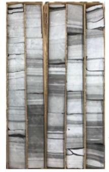
Clast-supported carbonate debrite
