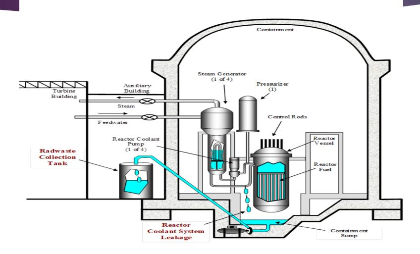
As long as any one of these barriers stays intact, significant amounts of radioactive fission products <u>CANNOT</u> be released outside the plant
