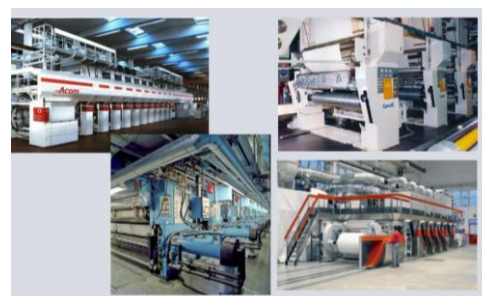
Figure 3: Rotogravure press for a packaging application [13].
