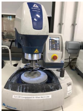
Figure 9: BUEHLER AUTOMET' 250 machine
