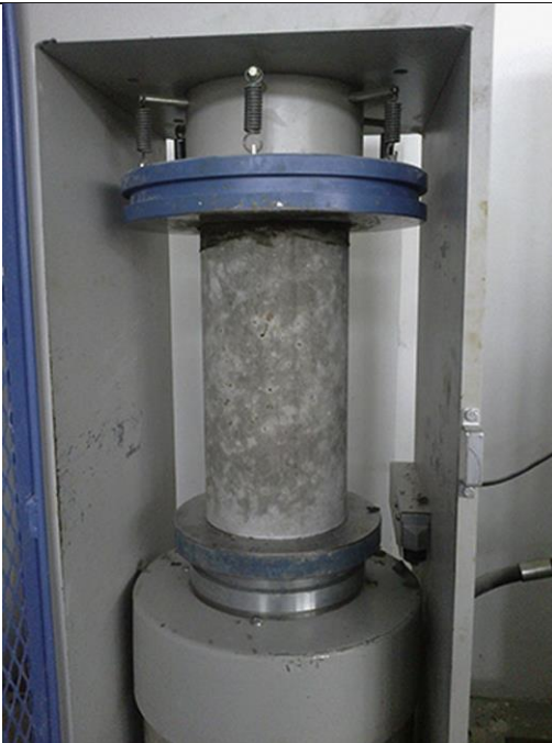
Fig. 1. Concrete compression test equipment.
