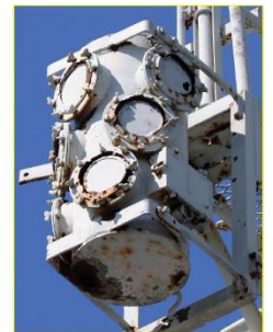
(Top) New "Nancy" beacons (yellow) and glass lenses (red) installed on upper superstructure. (Below) Close up of range finder window (l), replica Nancy beacons (c), and original beacon (r).
