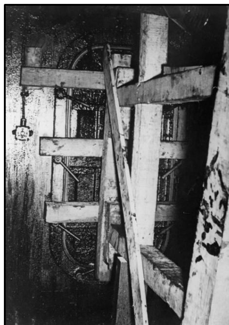
Shoring reinforces a watertight door damaged in the September 15 torpedo attack. The door leads into a washroom on the third deck.
