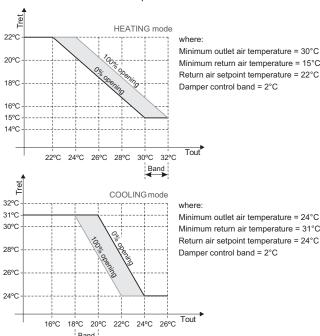
Minimum mixing air temperature. This value is established on the CU11a display, on 12°C in HEATING mode and 35°C in COOLING mode.
