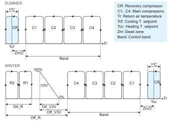
The recovery compressor can function even though there is no demand, depending on the temperature measured by the outlet air probe:
