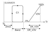
Tr: Inlet air temperature Tc: Cooling setpoint temperature Zm: Dead zone Band: Control band
