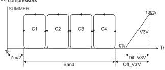
As support in COOLING mode, it is possible to incorporate a cold water coil (V3V). For the regulation of the coil, the control has a proportional or on/off output Y2 which controls the three-way valve.
