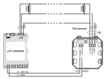
**Important:** It is recommended to insert an electrical resistance of  $120\Omega$ , between connectors TX+ and TX- of the  $\mu$ PC MEDIUM output (connector J10) and on the final component of the RS485 network, to avoid potential problems of communication.
