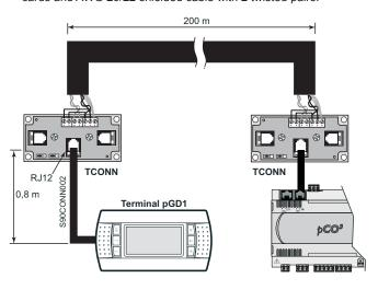
From 200 to 500 metres, it is necessary to use the TCONN bypass cards, AWG 20/22 shielded cable with 1 twisted pair and external 20...30Vdc (150 mA) power supply.
