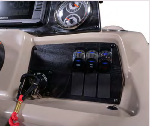
Key-start ignition, and light switches, all in one place.
