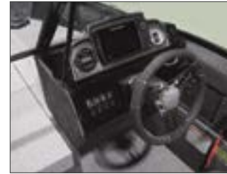
Bluetooth stereo, GPS fish/depth finder, and illuminated gauges and switches.
