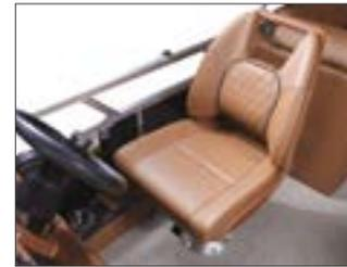
The swivel seat rotates 360° and slides forwards and back.
