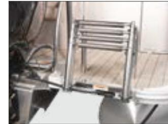
Telescopic stainless steel boarding ladder makes it easy to climb aboard from a dip in the lake.
