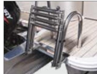
Large telescopic stainless steel boarding ladder makes it easy to climb aboard from a dip in the lake.
