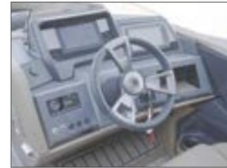
Brand new fibreglass helm with tilt steering, Bluetooth stereo, motor gauges, touchscreen GPS fish/depth finder.
