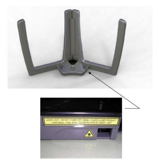
Warning Labels are located on side next to the USB connector as shown.
