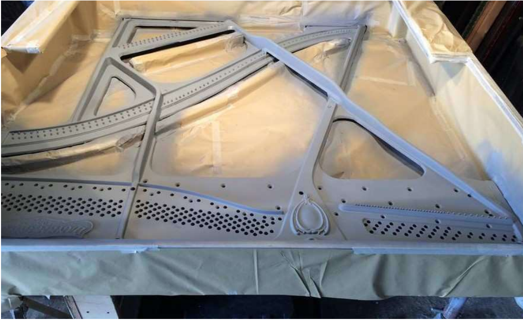
2 coats primer sprayed to frame
