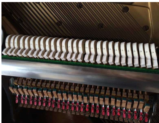
Bass hammers installed and aligned
