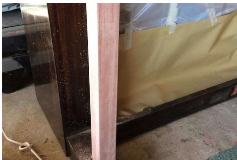
Left leg with completed veneer work
