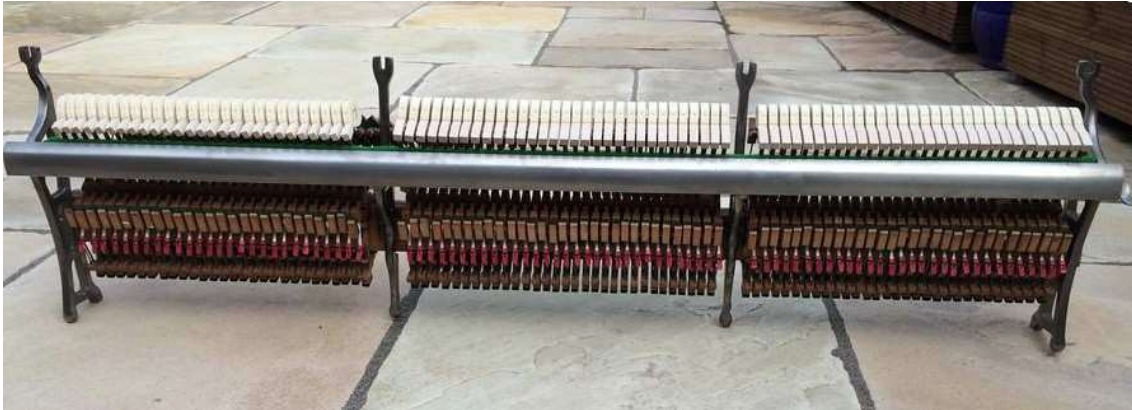
Completed action with new hammers installed
