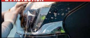
Did you know that 99% of the time the fading and oxidation of your headlight can be repaired like new without removing any parts. The exterior of the headlight plastic fades and oxidises and in bad cases it yellows and fine cracks appear an effect known as "crazing"
