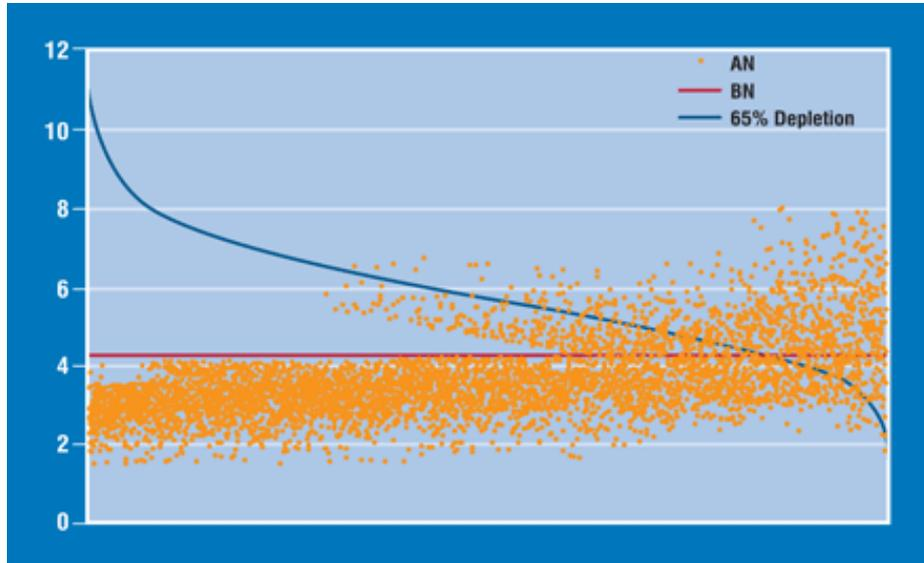
**Fig. 6.** Determining Optimal Drain Intervals Using Acid Number (AN)
