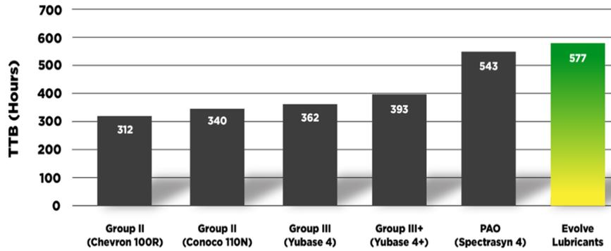
Fig. 7. Accelerated Oxidation Test. Wells, J. Novvi LLC, 2021
