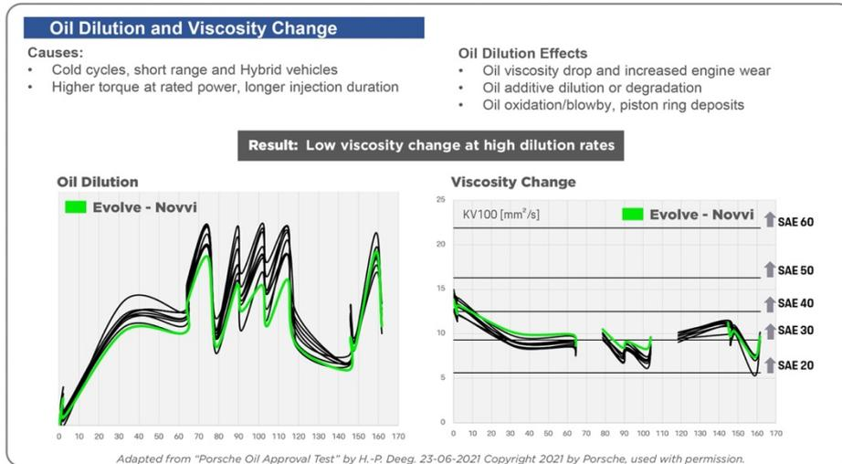
Fig. 2. Results for oil dilution vs. viscosity change. Wells, J. Novvi LLC, 2021
