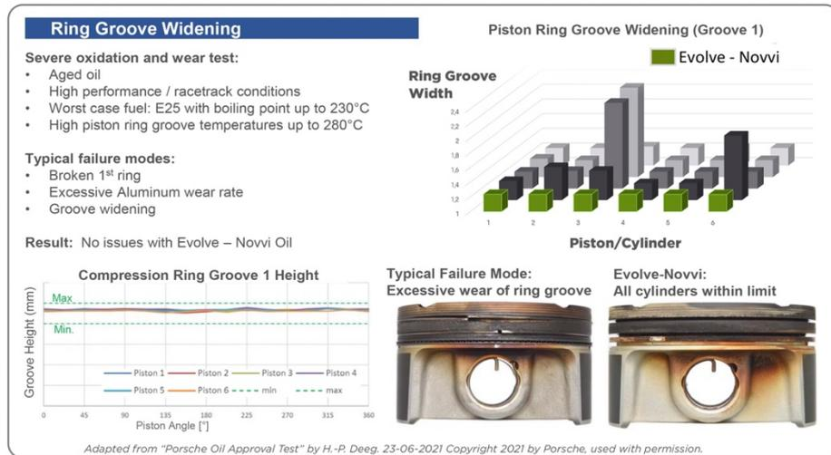
**Fig. 1.** Ring Groove Widening. Wells, J. Novvi LLC, 2021
