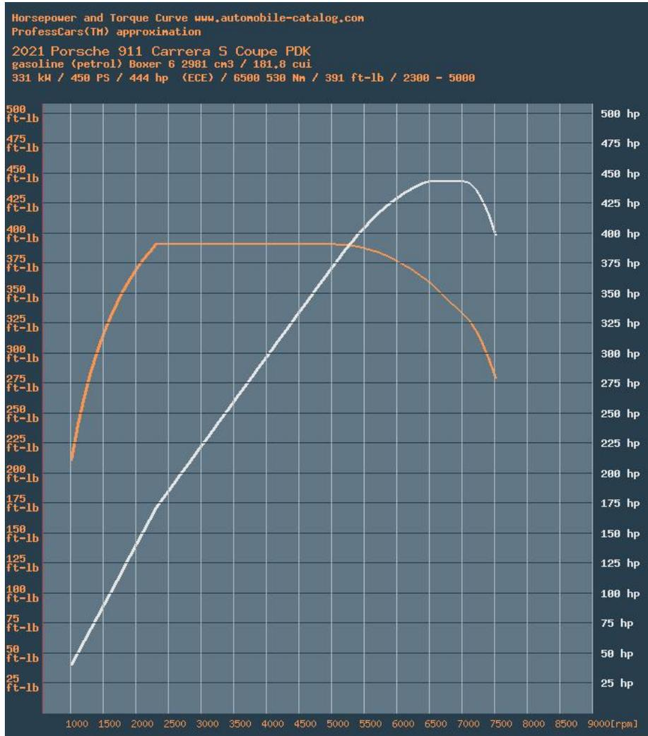
**Fig. 5.** 2021 Porsche 911 Carrera S Coupe PDK Horsepower and Torque
