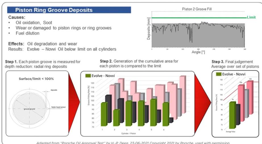
Fig. 3. Results Of Piston Ring Groove Deposits. Wells, J. Novvi LLC, 2021
