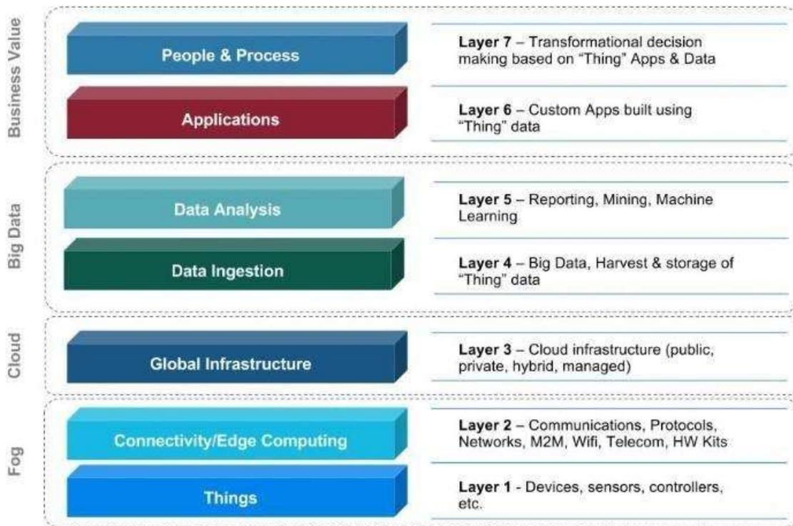
Figure 2: Seven Layers Architecture
