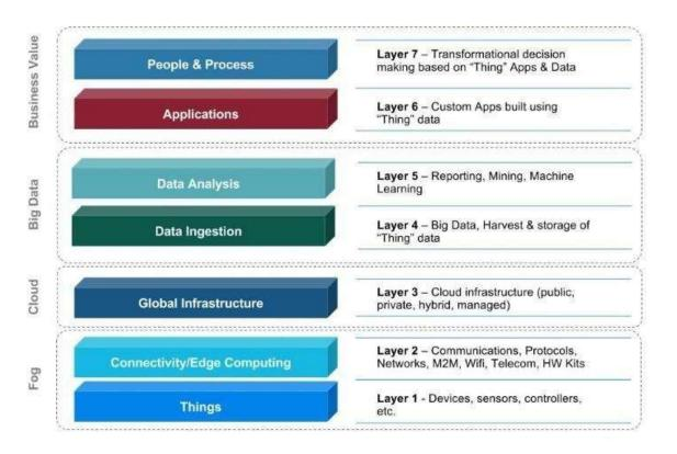
Figure 2: Seven Layers Architecture
